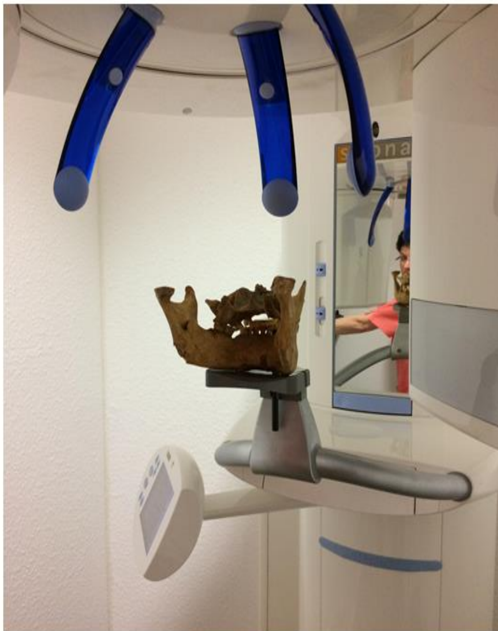
Figure 2. Sirona 2D/3D hybrid device Orthophos XG 3D in Dr. med. dent. George Gabbour Dental practice in Erfurt
